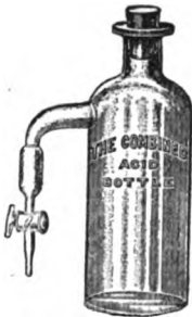
FIG. 14.—The combined acid bottle for rapid work.
